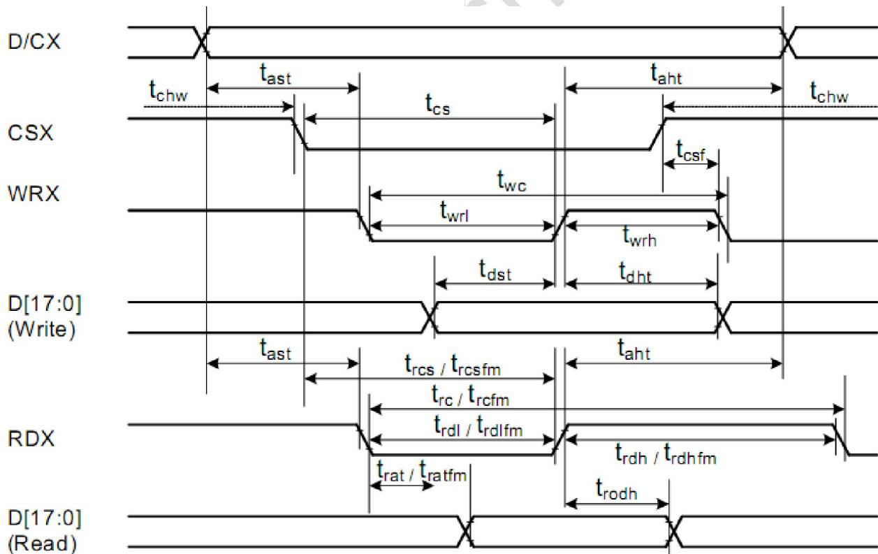
(Ta = 30 to 70 °C, IOVCC=1.65V to 3.3V, VCC=2.5V to 3.3V, VSS=0V)
