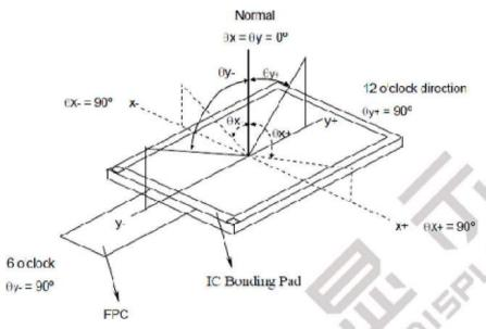
Note 6: Optical characteristic measurement setup.
