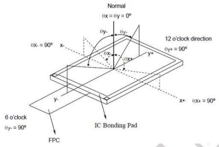
Note 8: Optical characteristic measurement setup.
