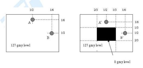
1 LA-LA'1/LA x 100%= 2% max., LA and LA' are brightness at location A and A'. 1 LB-LB'1/LB x 100%= 2% max., LB and LB' are brightness at location B and B'.
