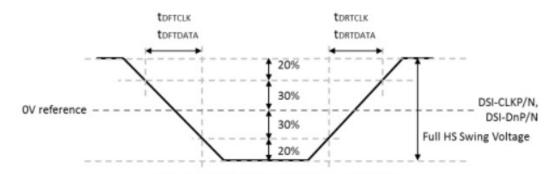
Figure 4-7 Rsing and Falling Timings
