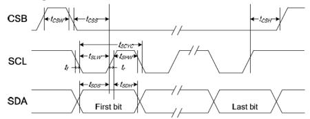
AGND = PGND =DGND = 0V, VDDA = VDDP= VDDI = 3.0 to 5.0V, Ta = 25°C
