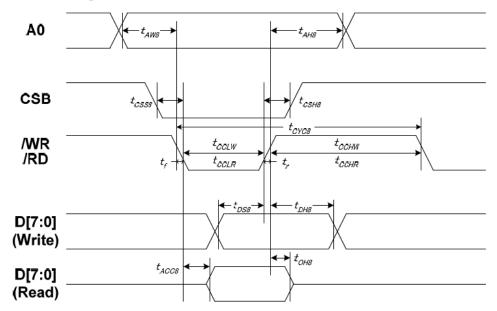
AGND = PGND =DGND = 0V, VDDA = VDDP= VDDI = 3.0 to 5.0V , Ta = 25°C
